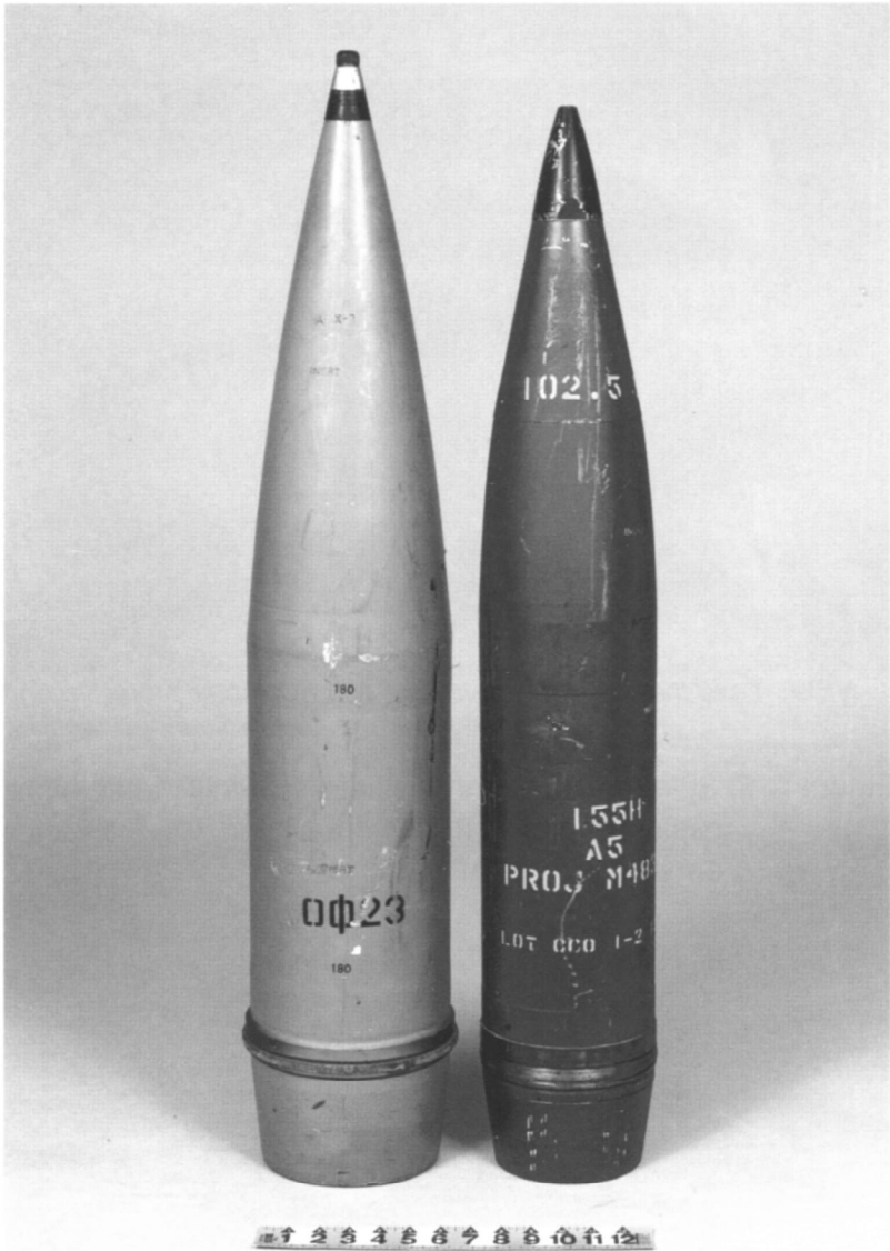
Figure C-4. Spin-stabilized projectiles, 180-millimeter (left) and 155-millimeter (right).
