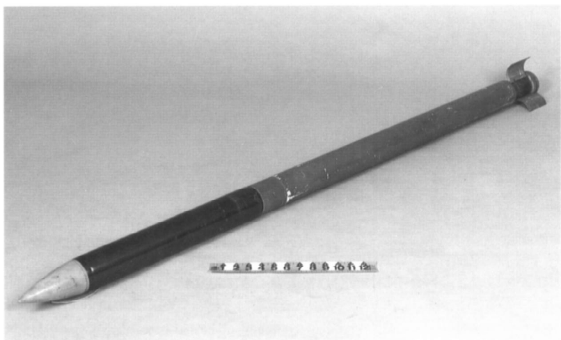
Figure C-18. Fin-stabilized rocket, 2.75-inch.
