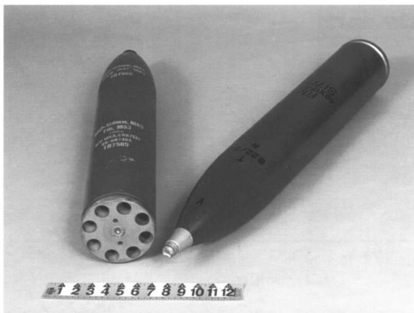
Figure C-14. Spin-stabilized rockets, 128-millimeter (left) and 132-millimeter (right).
