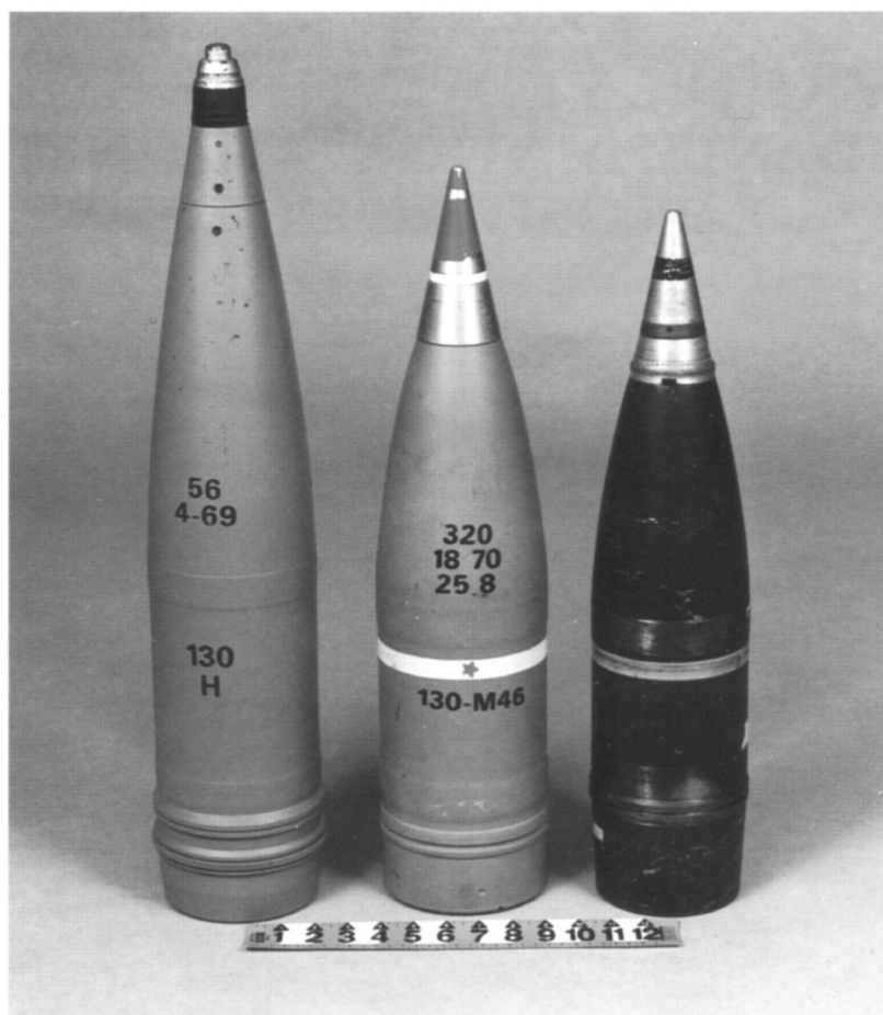
Figure C-2. Spin-stabilized projectiles, 130-millimeter.
