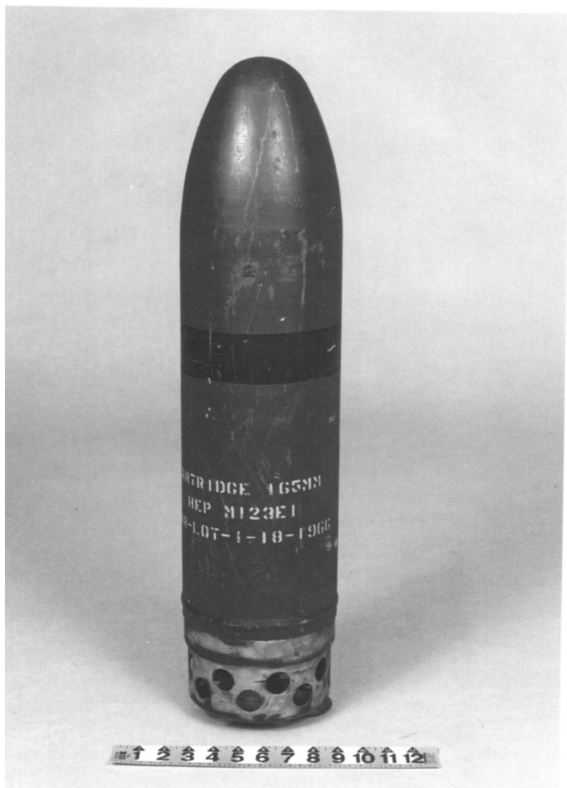
Figure C-6. Spin-stabilized projectile, 165-millimeter HEP.
