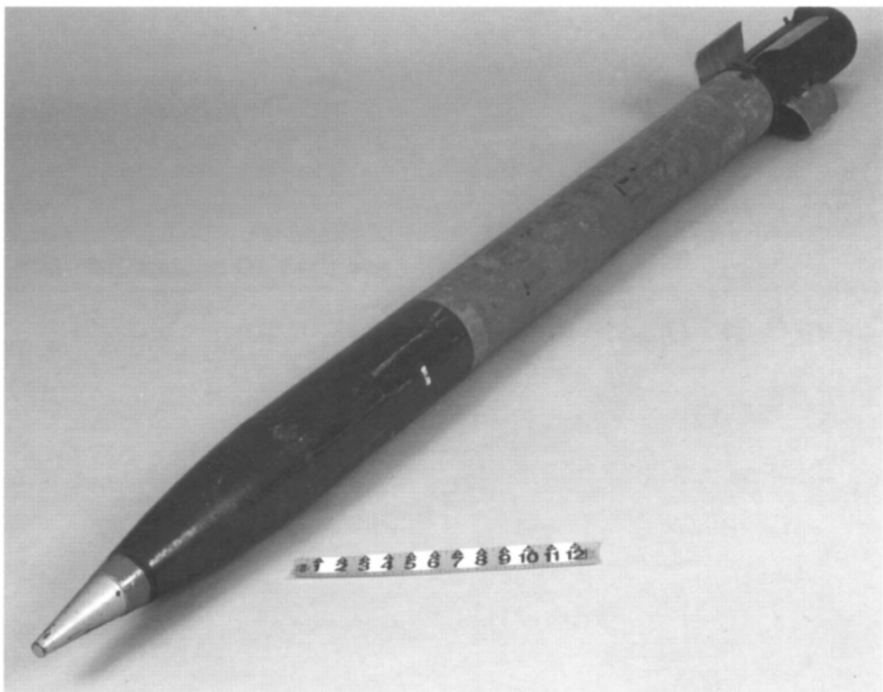
Figure C-20. Fin-stabilized rocket, 122-millimeter.
