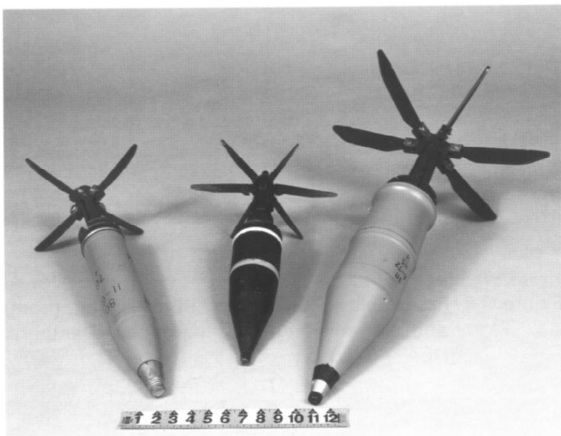
Figure C-9. Folding-fin stabilized HEAT projectiles.
