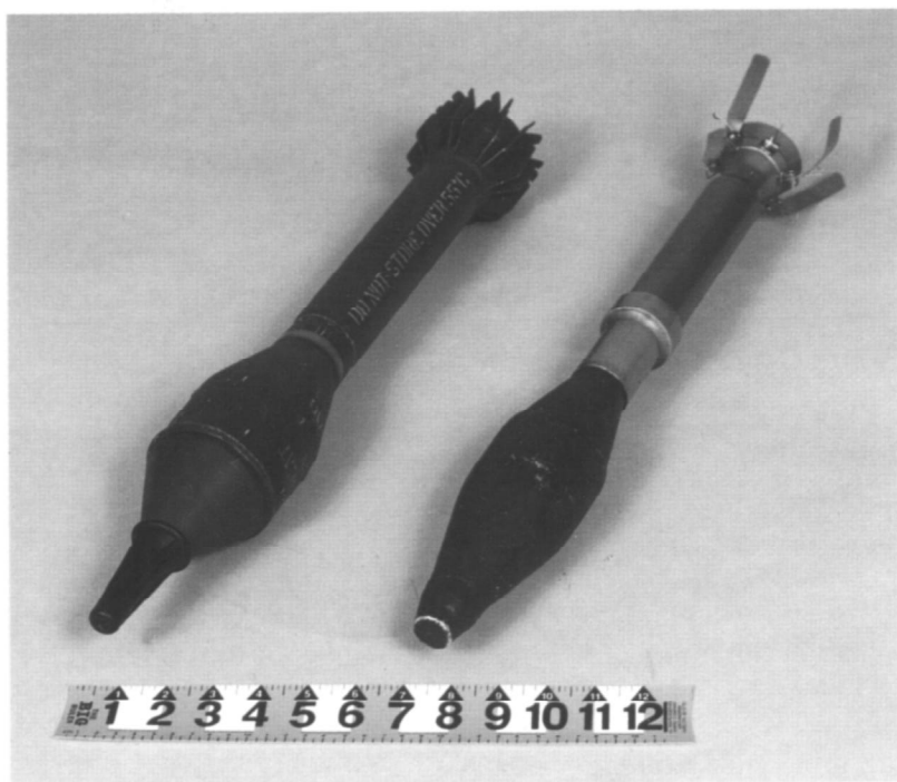
Figure C-15. Fin-stabilized HEAT rockets.
